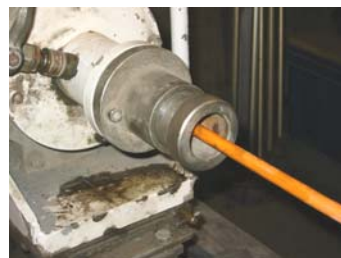
Fig.: Transfer cable of the overcoring probe led through the drilling head under tension
