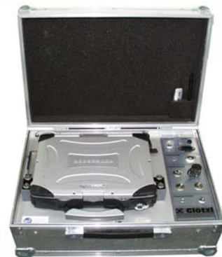
Fig.: Supply unit for overcoring probe
