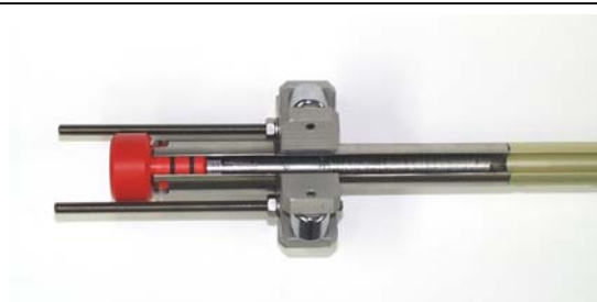
Figure: Settlement rods with depth stop and bayonet catch
