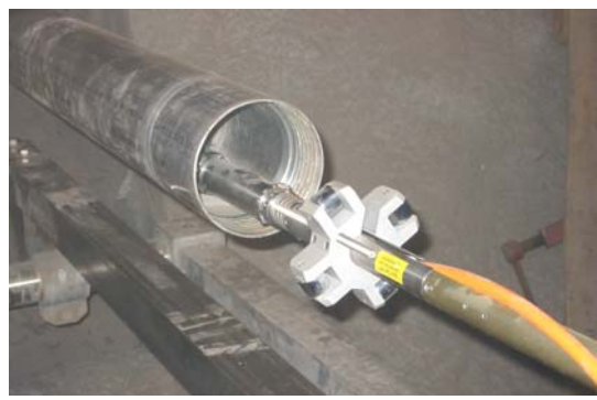
Figure: Installation of the overcoring probe
