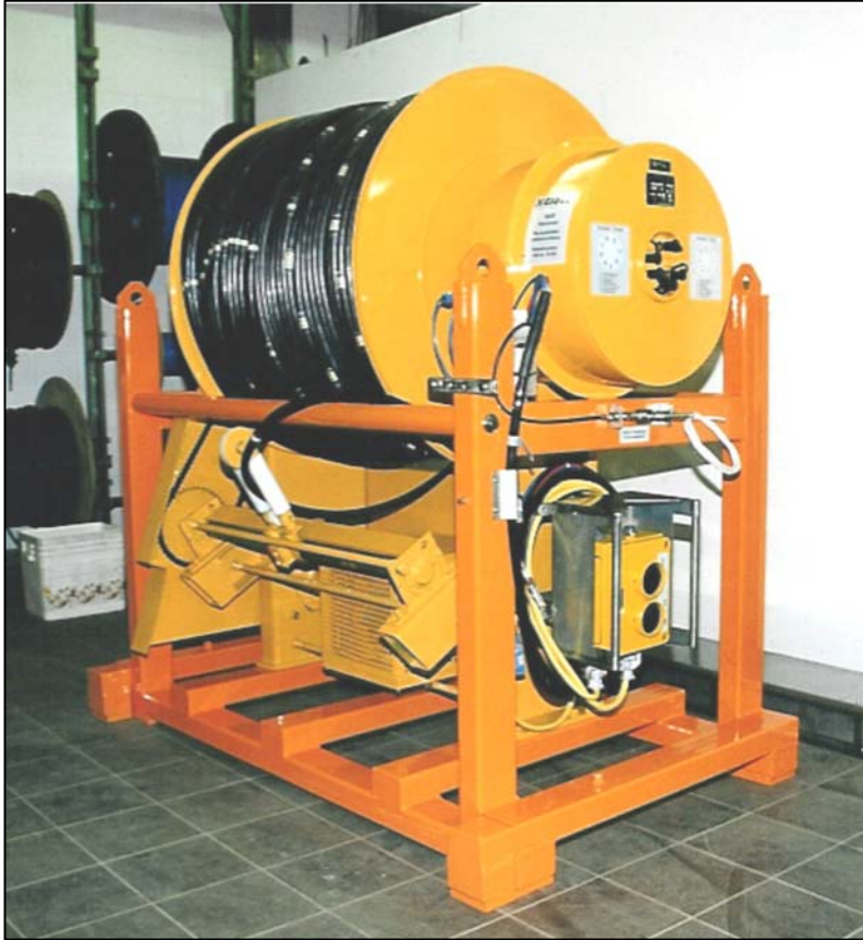
Figure: Cable reel of permeability measuring device
