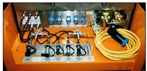
Figure: Data station connections
